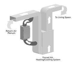
Fig. 3 Remote mount installation diagram.
