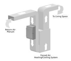
Fig. 2 Return air installation diagram.
