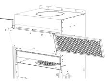
Fig. 6 Slide out PCO filter.
