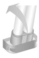
Fig. 4 UV lamp installation.
