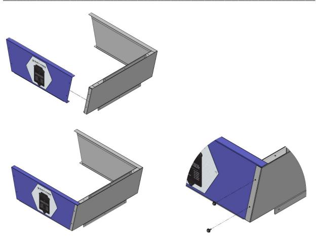
Figure 5: Remaining side and rear panel alignment and assembly.
