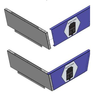
Figure 3: Side and rear panel alignment and assembly.
