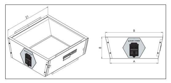
Figure 2: Side Access Unit dimensions.
