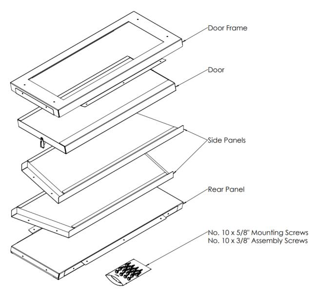
Figure 1: Components included inside the box.
