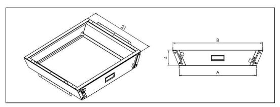
Figure 3: Closet Access Unit dimensions
