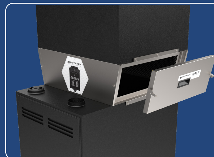
The SST2 installs between the furnace and the coil to provide more efficient airflow between different-sized components.
